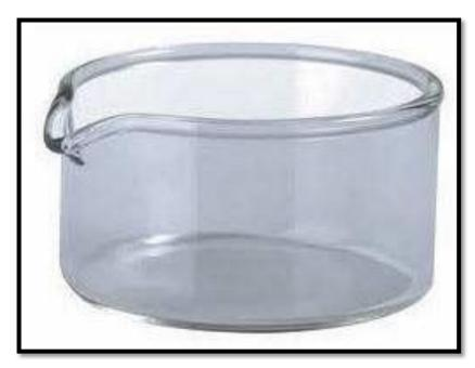
Figure 1.13 Crystallization dish
