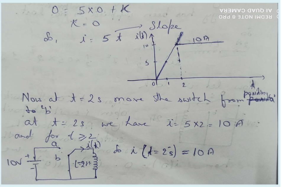
MOM,  $\Gamma \frac{dy}{di} = 0 \Rightarrow 5 \frac{dy}{di} = 0$  AREMAD DAUD IA this means of L'amost be constant for \$ 22 Energy istored in the inductor at 1 > 2  $W = \frac{1}{2} \times Li^2 = \frac{1}{2} \times 2 \times 100 = 100 \text{ J}$
