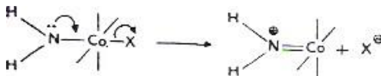
Fig. 6.5: Stabilization of the intermediate 5-coordinate species through the resonance effects involving \text{NH}_2 group.
