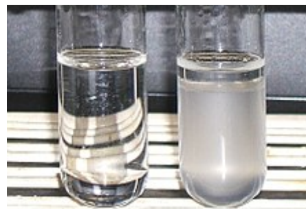
Lucas test: negative (left) with ethanol and positive with t -butanol
