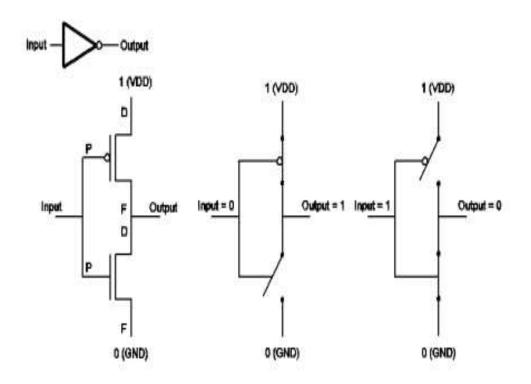
We have just seen how to implement a simple logic gate using transistors. To implement the rest of logical gates (and whatever circuit we might think off), we will analyze first the behavior of the transistors when connected in a "series" fashion or in a "parallel" way.
