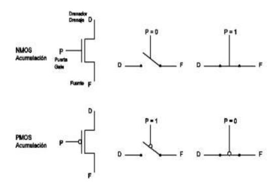
When a circuit contains both NMOS and PMOS transistors we say it is implemented in CMOS (Complementary MOS).
