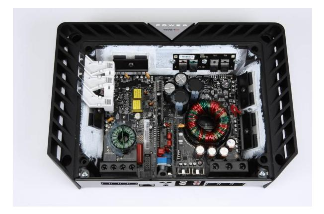
The inside of a <u>Rockford Fosgate T500-1bdCP</u> showing the transformer (the coil of red and green wires) and output transistors (black rectangles glued to the heatsink with white thermal paste).
