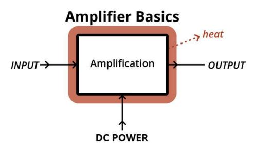
**Amplifier Class** is the system for combining power and signal. Amp class differs from amp to amp with efficiency and sound fidelity dependent on which design gets used. In all designs, banks of output transistors, each a little amp by itself, add their collective power together to provide the amplifier's final output.
